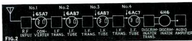
Fig. 2—Block diagram of F-M receiver showing necessary connection points to facilitate i.f. alignment
